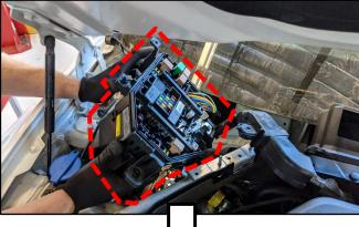
8b. Remove cable band (E) secured to the junction box.
