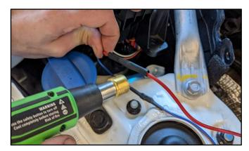
16. Insert/lock the two (2) ESC wires onto the junction box in the new location shown.
