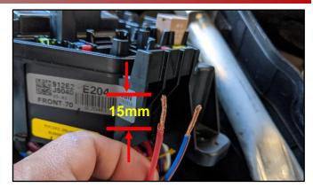
Join the lead wire from the kit to the ESC wire end and crimp the two wires together
