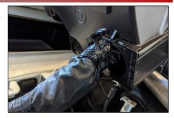
18. Install the two (2) new supplied 25 Amp fuses (J) from the wire kit in the location shown.
