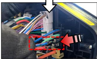
12. Cut off the two (2) ends of the detached ESC wire terminals and strip off the insulation of the two (2) wire ends (approximately 15mm as shown).
