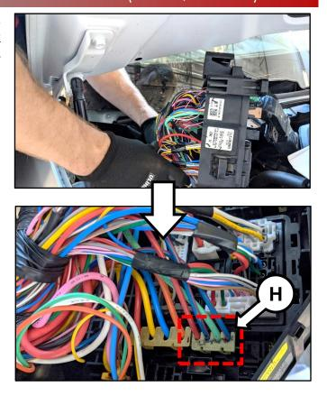
10. Using a pin remover (I), unclip the two (2) ESC wire terminals from the top of the junction box.
