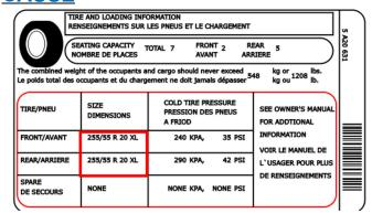
During vehicle production, a tire pressure label containing the incorrect tire size was installed to the vehicle "B" pillar.
