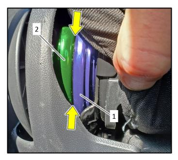
Inboard Recline Mechanism (closest to the center tunnel):
