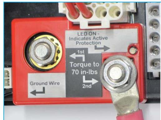
(3.7) Turn on Main Power Switch and verify that the LED illuminates.
