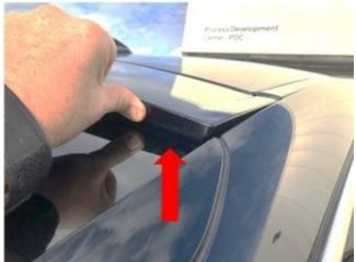
3. While pressing upwards using a thumb and moderate force, measure the gap between the glass and the bottom of the rear spoiler (arrow) again.
