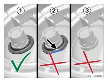
Figure 1: connecting flange of fuel-pump unit
