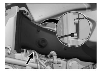
• Check that the throttle-valve cable is seated in the guide of the air intake pipe **(arrow)** and that it is has not been pulled out of the divider.
