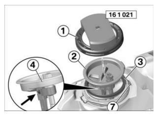
Installing additional fuel-pump flange
