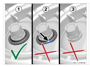
Figure 1: connecting flange of fuel-pump unit
