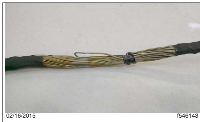
Fig. 6, Overlay Added to the Damaged Area of the Harness
