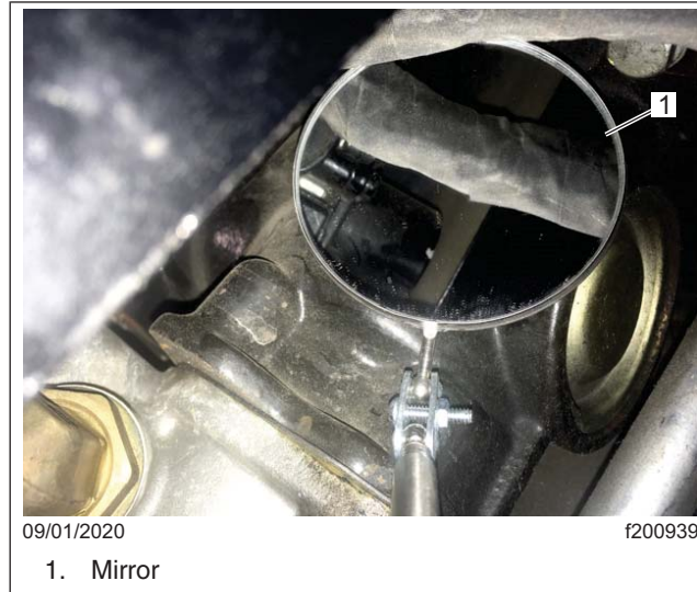
Fig. 2, Inspection by Mirror
