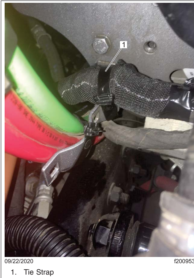
Fig. 13, Securing the Harness using Tie Strap
