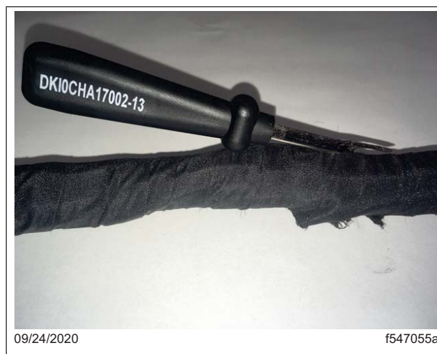
Fig. 18, Cutting the Fiber Using the Blunt End of the Seam Ripper
