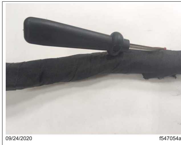
Fig. 17, Cutting an Opening into the Fiber Wrap
