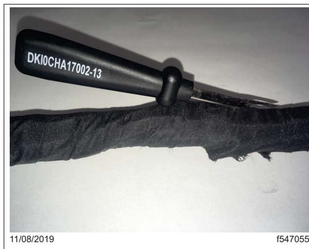
Fig. 4, Cutting the Fiber Using the Blunt End of the Seam Ripper
