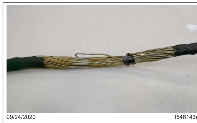
Fig. 20, Overlay Added to the Damaged Area of the Harness
