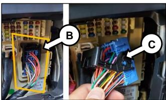
Locate the white wire with orange tracer 5. (Pin 10 of the ICU-C) connector (B) and use the provided joint connector (D). Install the provided joint connector (D) over the white wire with orange tracer. Next, insert the supplied wire 3/4" into the open cavity on the joint connector.
