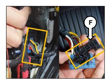
9. Locate the blue wire (G) (circuit Pin 7) of the FF12 connector and cut the wire about 4"- 5"inches from the back of the connector.
