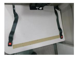
5. Remove outside bolts from female tether portion of seatbelt and replace with a new 24" tether. Tighten to 30ft.-lbs. (Repeat on other side.)
