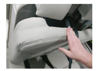
2. Extend the seatbelt all the way out. Measure from the bracket flat along the seat base to end of extension.
