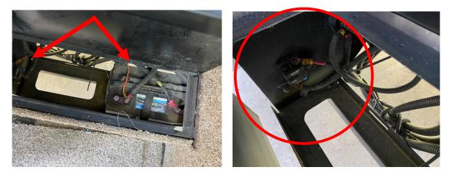
3. If the breaker is 100 amp breaker, it will need to be replaced with a 70 amp breaker. Continue to Step 4.
