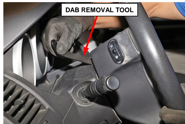
Figure 2 – DAB Removal Tool
