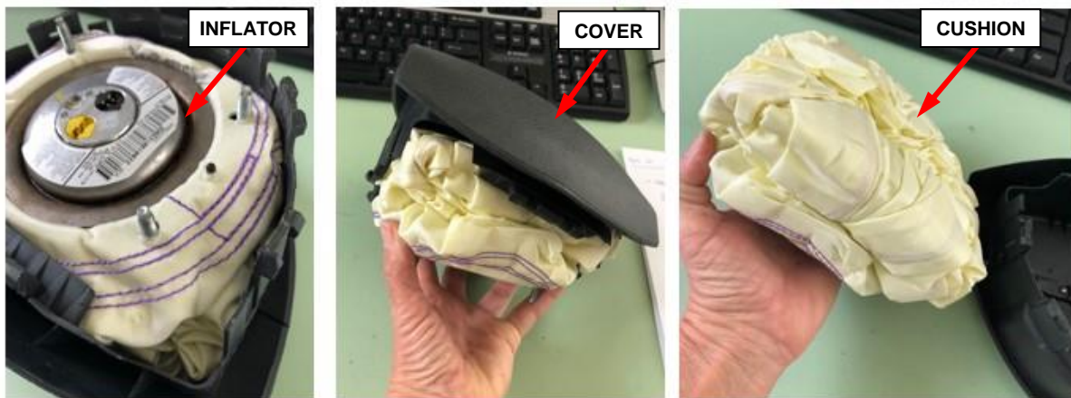
Figure 13 – Remove Cover from Cushion
