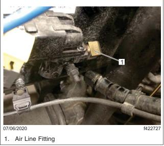
Fig. 8, Loosening the Brake Chamber Air Line Fitting
