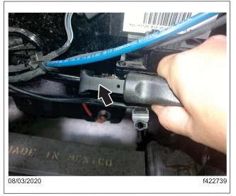
Fig. 5, Disconnecting the Plastic Air Line
