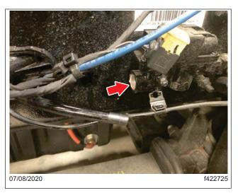
Fig. 6, Disconnecting the Quick Connect Fitting
