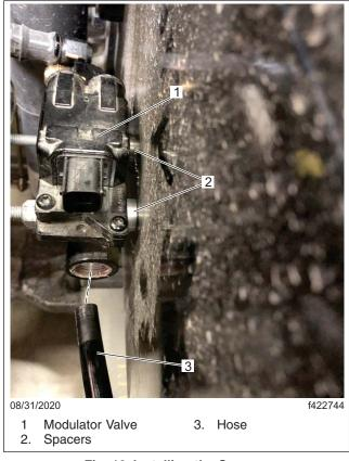
Fig. 10, Installing the Spacers
