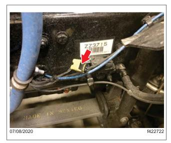
Fig. 2, Electrical Connector
