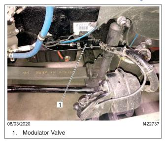
Fig. 1, Locating the Modulator Valve
