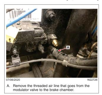
Fig. 7, Removing the Threaded Air Line
