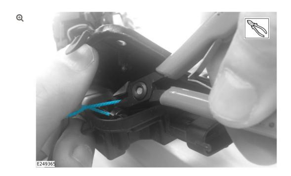
Use a suitable tool to cut the keyless vehicle motor cord.
