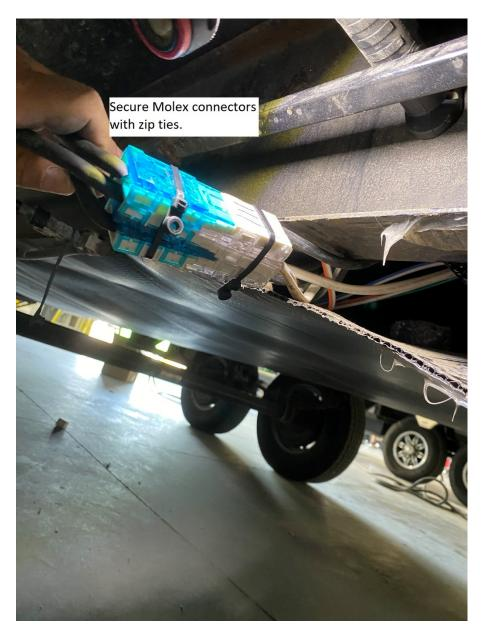
Step 5: Secure the Molex connectors off the underbelly.
