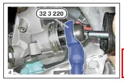
e. Remove the tie rod assembly from the steering shaft of the steering gear assembly using SST.
