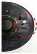
Reassemble the front wheel, pay attention to the front wheel speed sensor, the front shock mount is inserted into the U-shaped slot at the white dot mark and/or the R engraved in card.
