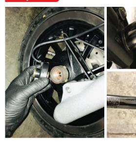
Remove the axle screw to drop front wheel. Separate ABS cover from sensor ring. (14mm bolt head and 19mm nut)
