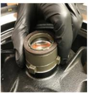
Remove the damaged speed sensor magnetic ring. Install the new magnetic ring from the recall kit. Screw-on the sensor snug-tight by hand.
