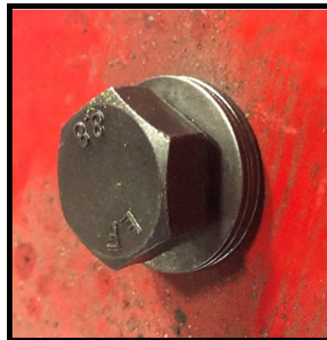
Figure 3 Bolt and Washer Correctly Attached and Torqued
