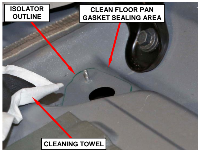
Figure 49 – Clean Gasket Sealing Area
