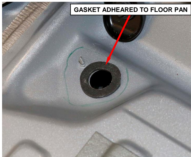
Figure 51 – 12-Volt Isolator Gasket
