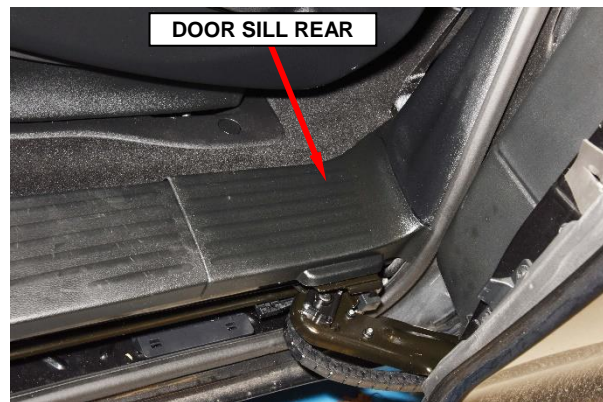
Figure 22 – Door Sill Rear
