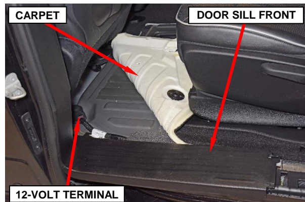
Figure 23 – Door Sill Front and Carpet
