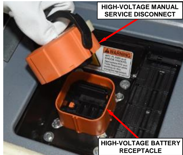
Figure 9 – High-Voltage Manual Service Disconnect and Receptacle
