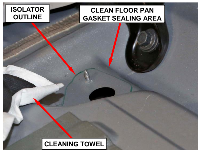
Figure 49 – Clean Gasket Sealing Area
