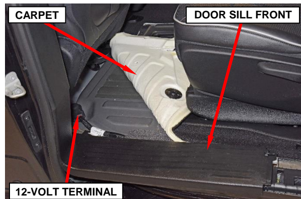
Figure 23 – Door Sill Front and Carpet
