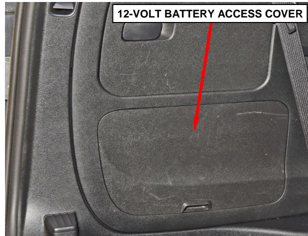
Figure 3 – Battery Access Cover
