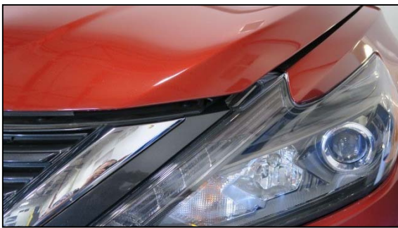
Figure 1 – Hood Open (primary unlatched)
