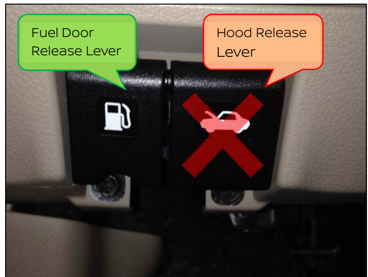
Figure 3 – Fuel Door & Hood Release Levers
