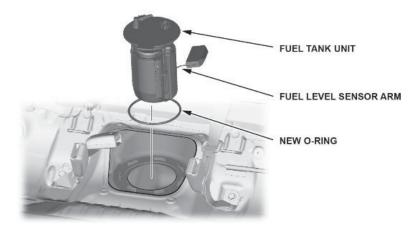
11.2. Line up the tab of the fuel tank unit as shown, and temporarily insert the new fuel tank unit cam lock ring.
