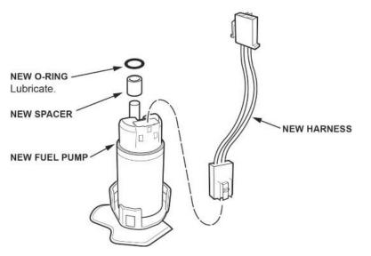
10.2. Install the fuel pump to the fuel filter.
