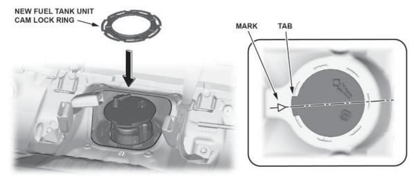
12. Lock the fuel tank unit cam lock ring.
