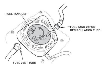
17. Tighten the fuel tank unit cam lock ring.
