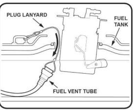
12.5. Remove the fuel tank unit with the O-ring.
