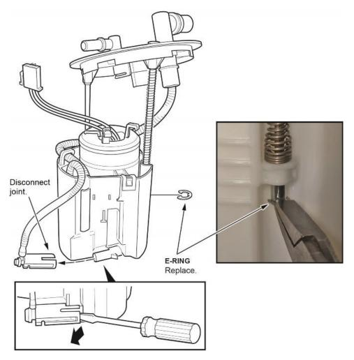
13.5. Disconnect the joint at the bottom of the reservoir.
