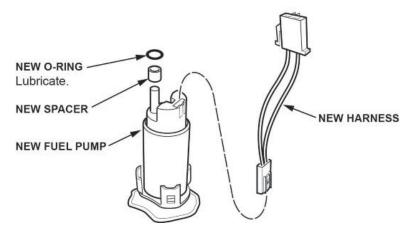
9.2. Install the fuel pump to the fuel filter.
