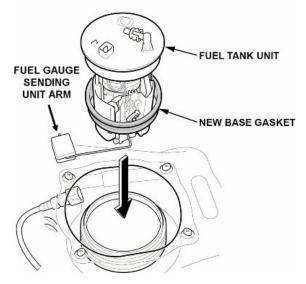
10.2. Line up the marks on the fuel tank and fuel tank unit, then insert the fuel tank unit into the fuel tank.
