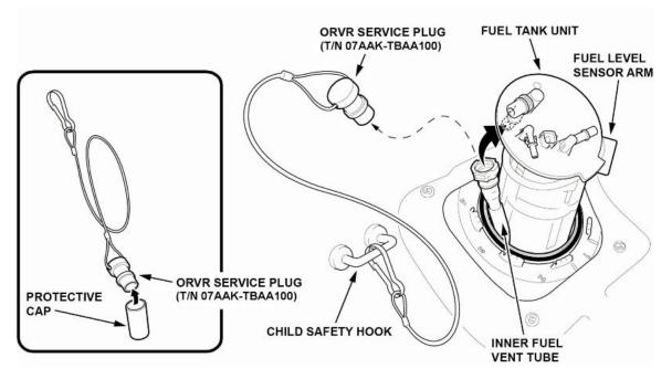
14.6. Remove the ORVR service plug from the child safety seat hook, and install the provided protective cap.
