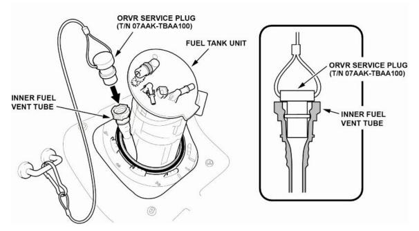
11.3. Install the ORVR service plug to the inner fuel vent tube. Make sure the ORVR service plug is fully seated by holding the inner fuel vent tube, and gently pulling on the plug's lanyard.
