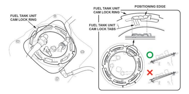
16.2. Turn the fuel tank unit cam lock ring clockwise using the fuel sender wrench.
