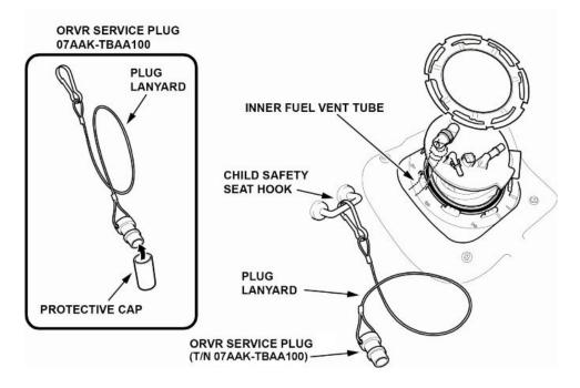
11.2. Disconnect the inner fuel vent tube from the fuel tank unit, and hold it. Do not allow the inner fuel vent tube to drop into the fuel tank.
