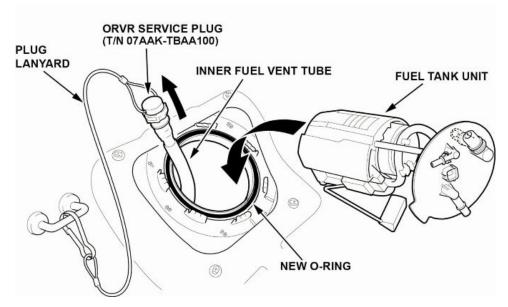
14.2. Grab the plug lanyard, and pull the inner fuel vent tube up until it is close to the fuel tank opening.
