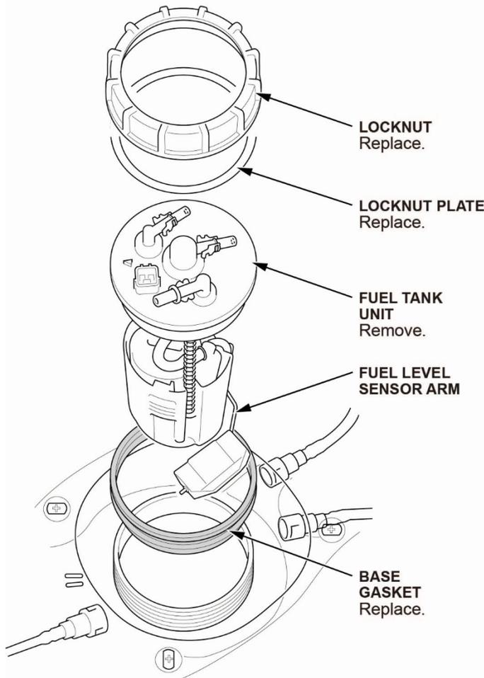
19. Disassemble the fuel tank unit.
