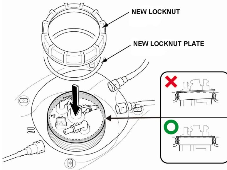
22.2. Tighten the fuel tank unit locknut to the specified torque using the fuel sender wrench.
