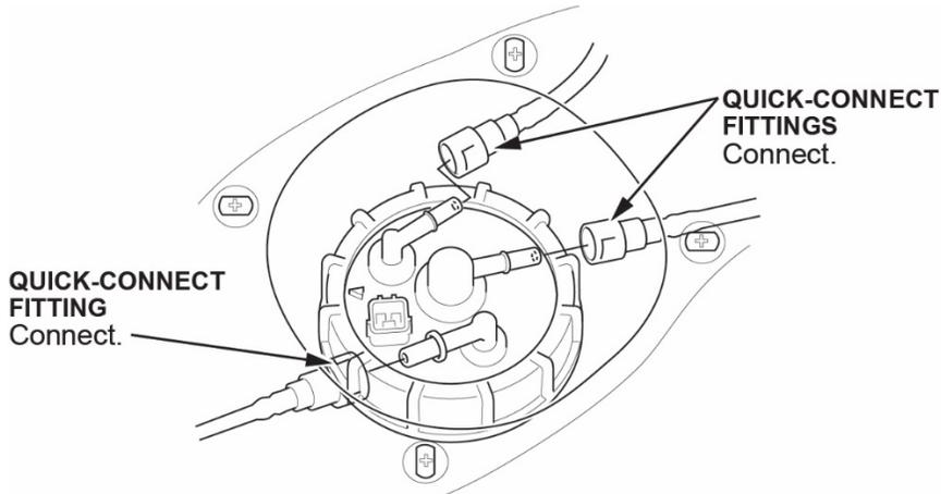
25. Connect the fuel tank unit connector.
