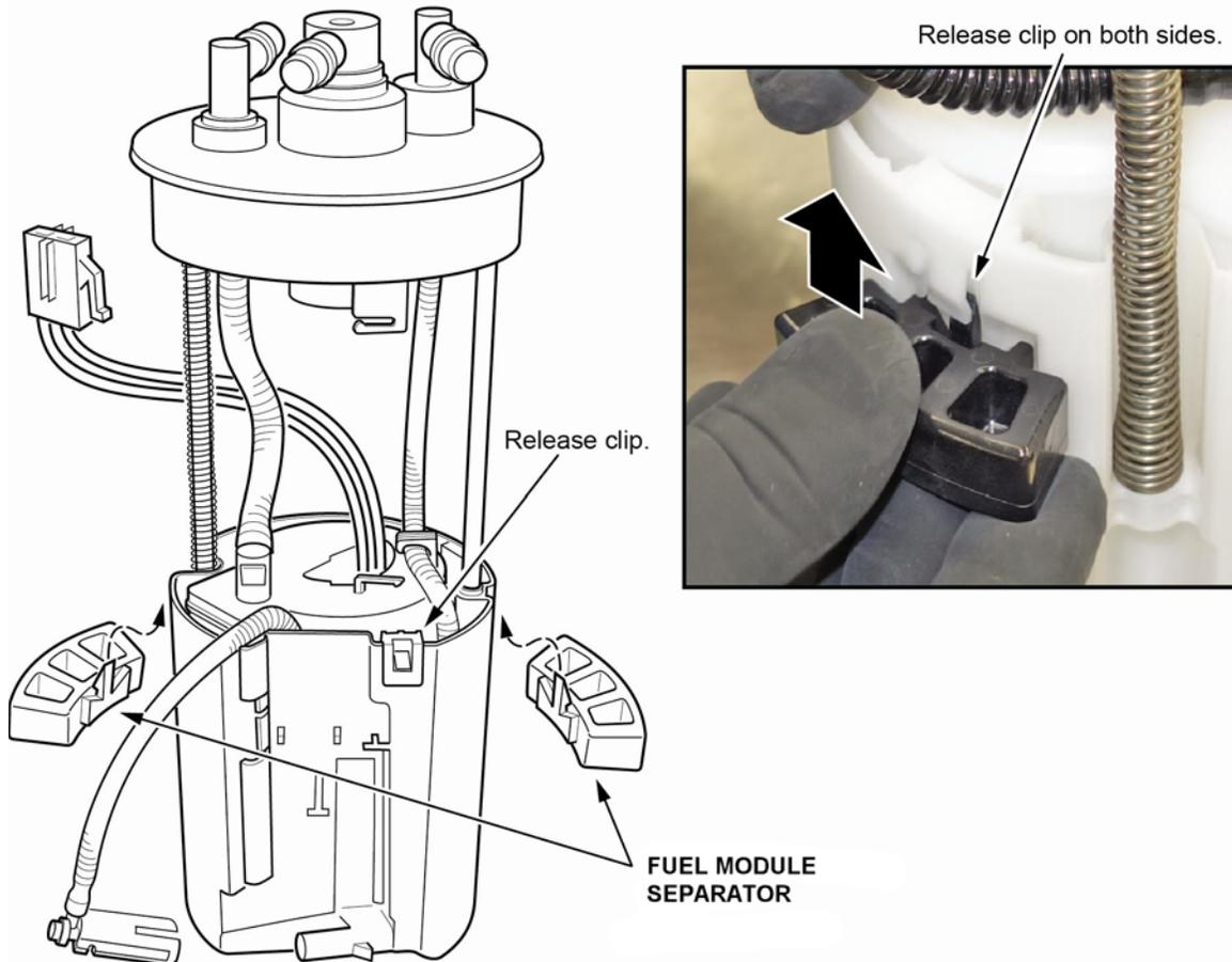
19.7. Remove the fuel pump assembly from the fuel filter.
