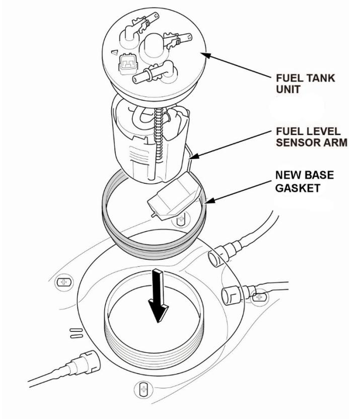
21.2. Line up the marks on the fuel tank and fuel tank unit as shown, then insert the fuel tank unit.
