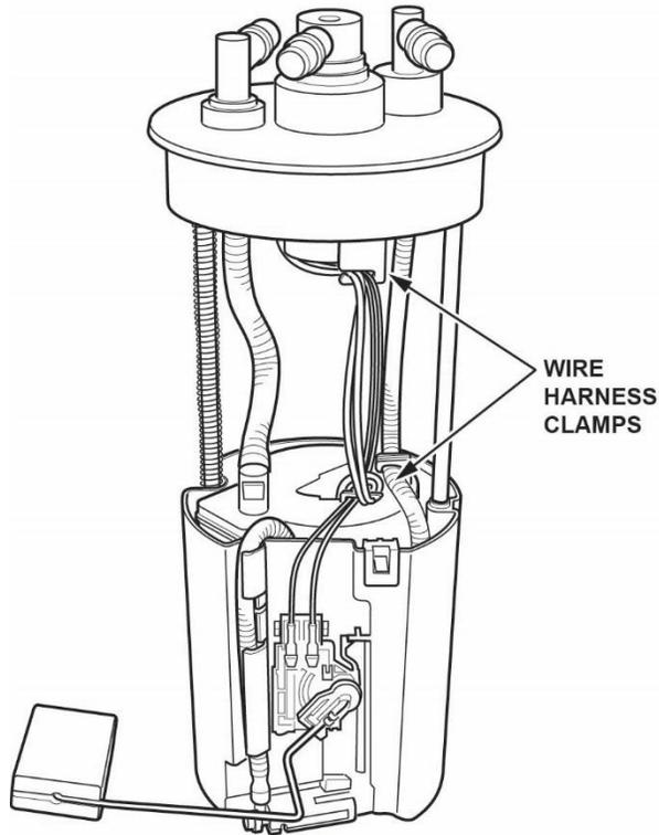
19.3. Remove the fuel level sensor.
