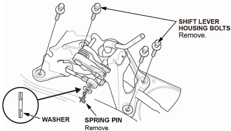
13.2 Remove the shift lever housing bolts.
