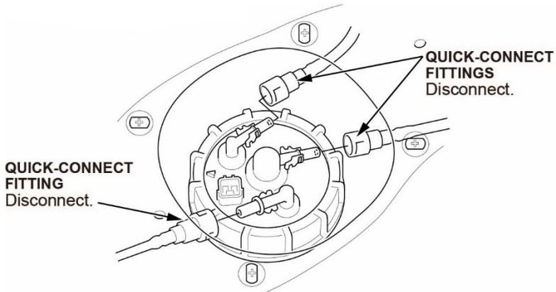
17. Loosen the fuel tank unit locknut using the Fuel Sender Wrench (T/N 07AAA-S0XA100).
