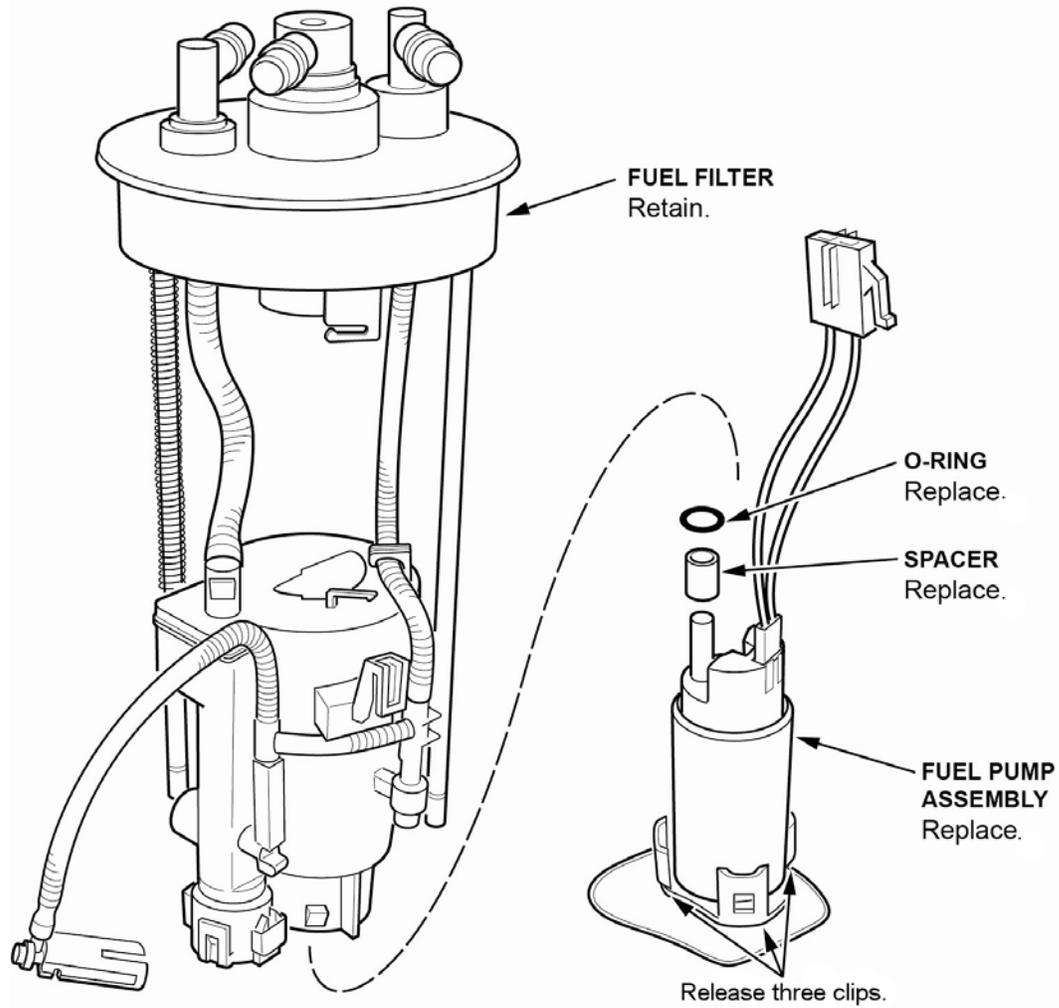
20. Assemble the fuel tank unit.
