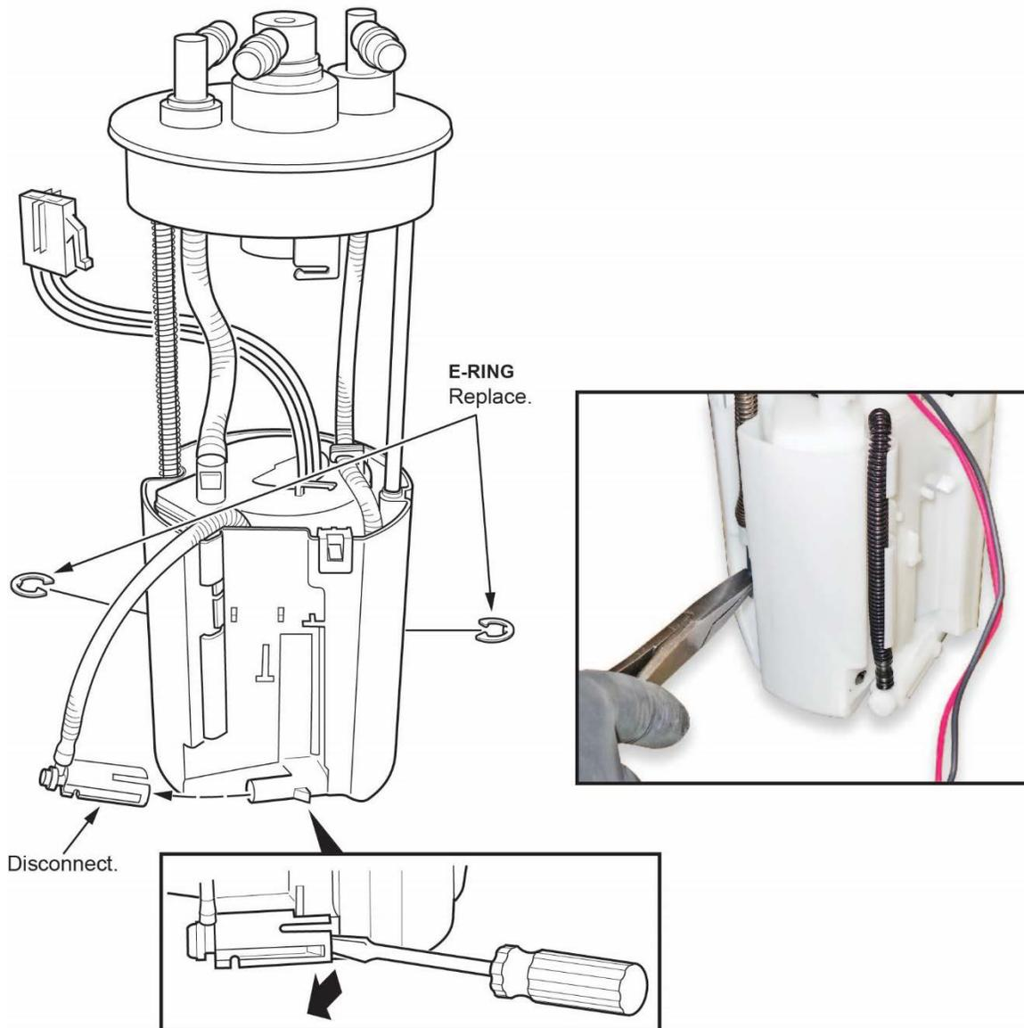
19.5. Disconnect the joint at the bottom of the reservoir.
