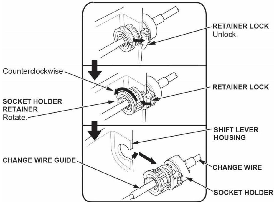
13.4 Rotate the socket holder retainer counterclockwise until it stops, then push the retainer lock into the socket holder retainer to lock the retainer.
