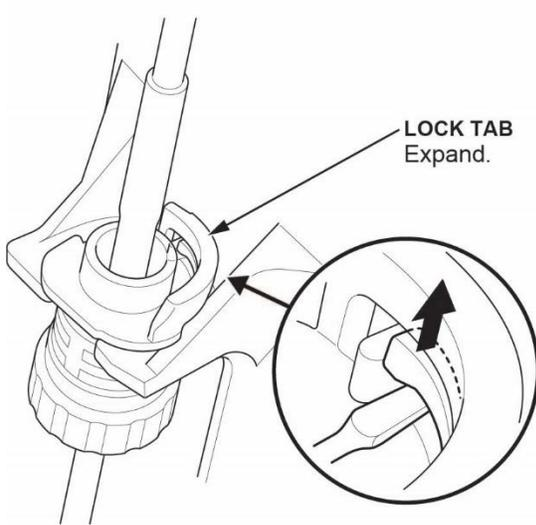
14.5 Rotate the socket holder retainer counterclockwise until it stops, then remove the shift cable.
