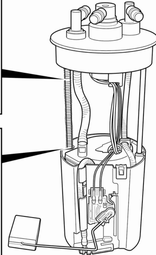
20.7. While compressing the fuel tank unit, make sure the movement is smooth and the fuel tube and wiring harness do not pinch or bind.
