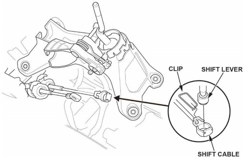
13.7 Disconnect the shift cable from the shift lever.
