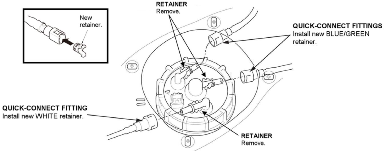
24. Connect the quick-connect fittings to the fuel tank unit.
