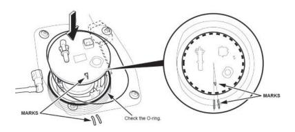
11. Tighten the fuel tank unit locknut.
