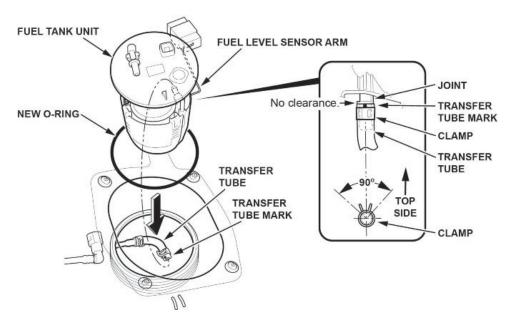
10.2. Align the marks on the fuel tank and fuel tank unit, then insert the fuel tank unit into the fuel tank.
