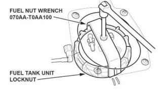
7. Remove the fuel tank unit locknut, and lift it up just enough to disconnect the transfer tube. Then, remove the fuel tank unit.
