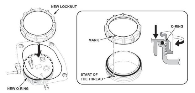
12. Tighten the fuel tank unit locknut to the specified torque using the fuel sender wrench.
