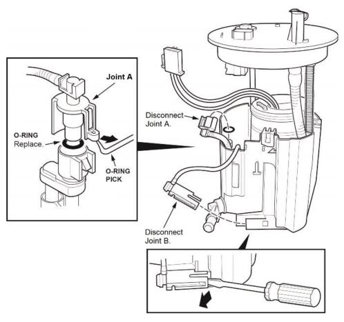
8.6. Disconnect Joint B from the bottom of the reservoir.
