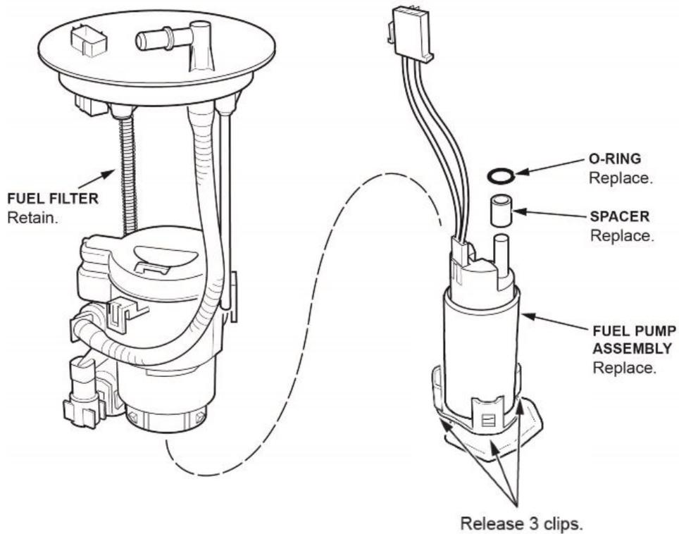
10. Assemble the fuel tank unit.
