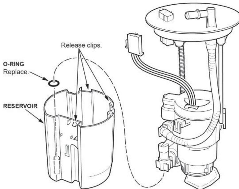
9.6. Remove the fuel pump assembly from the fuel filter.
