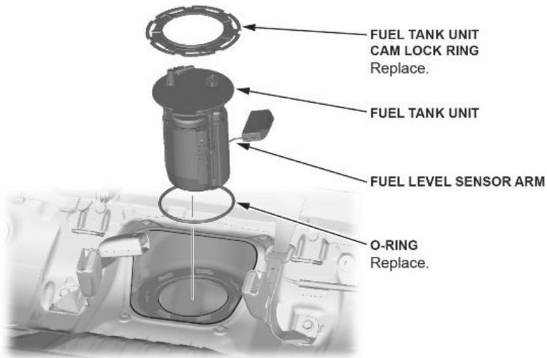
9. Disassemble the fuel tank unit.
