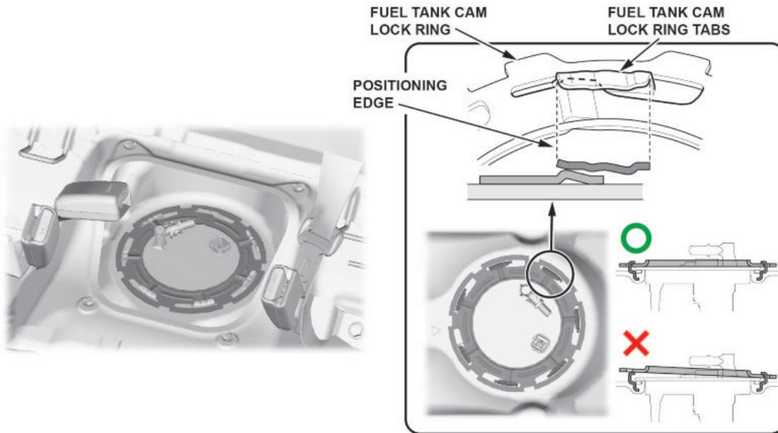
12.2. Turn the fuel tank unit cam lock ring clockwise using the fuel sender wrench.
