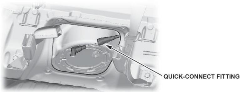
15. Connect the fuel tank unit connector.
