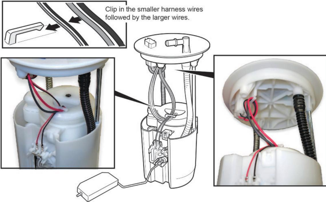
10.7. While compressing the fuel tank unit, make sure the movement is smooth and the fuel tube and wiring harness do not pinch or bind.
