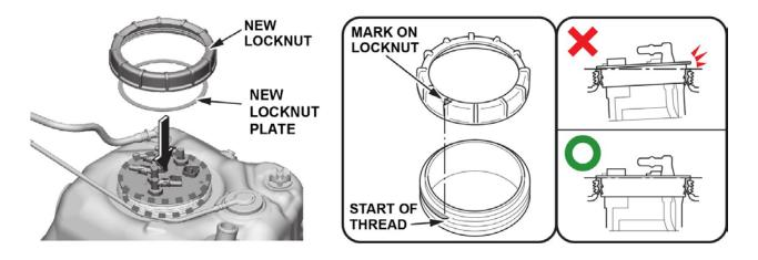
36. Tighten the fuel tank unit locknut to the specified torque.
