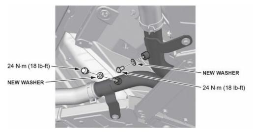
20. Disconnect the water hoses from the center pipes, and cap off the ends. Replace the water outlet hose during installation.
