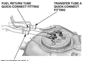
TRANSFER TUBE A QUICK-CONNECT FITTING
