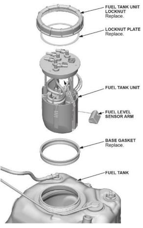
34. Partially insert the new fuel tank unit into the fuel tank with a new base gasket.
