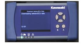
Confirm the downloaded vehicle ECU data on the Completion of Vehicle ECU Data screen.
