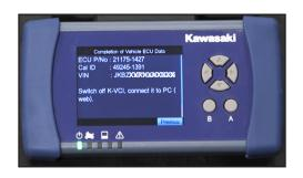
Slide the mode switch of KVCI device to the OFF position.
