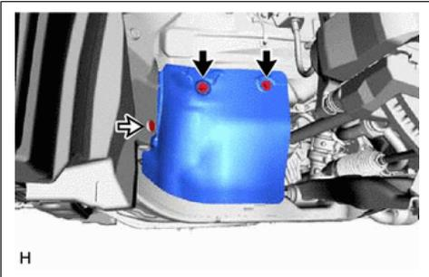
**10. REMOVE FRONT FENDER APRON SEAL LH & RH**
