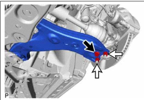
**11. REMOVE SUSPENSION ARM ASSEMBLY LH & RH**
