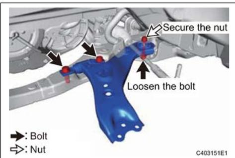
b. Remove the 3 bolts, nut and front lower No. 1 suspension arm sub-assembly from the front frame assembly.
