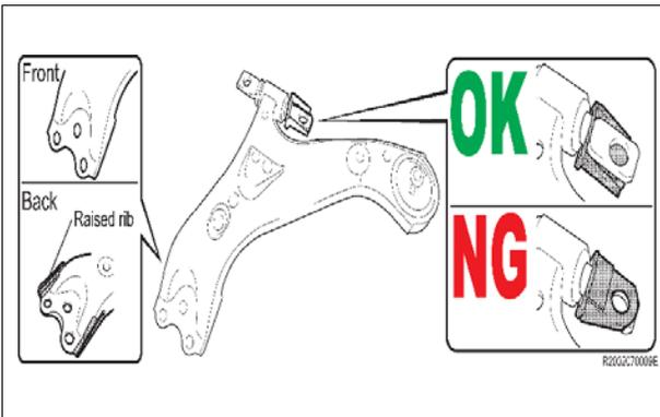
2. INSTALL THE **NEW FRONT LOWER NO. 1 SUSPENSION ARM SUB-ASSEMBLY (LH & RH)**
