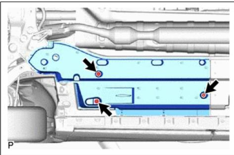
b. Loosen the 3 nuts and remove the front floor cover RH from the body.
