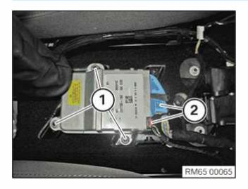
**Installing the airbag control unit** Further information is available.
