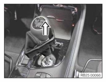
• Use wedges (1) to unclip the gaiter and pull it off upward.
