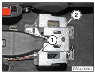
• Loosen the nuts (1) and remove the holder (2).
