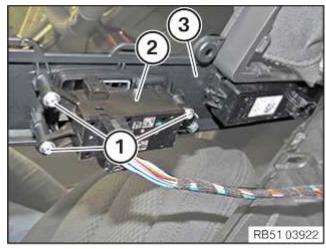
Removing the front storage compartment
