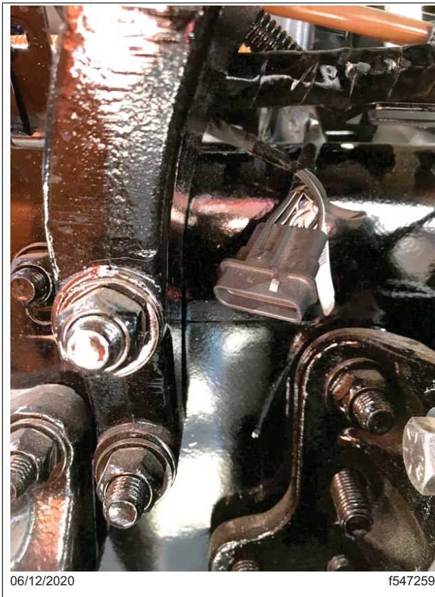
Fig. 6, Splice Pack with Cover Removed
