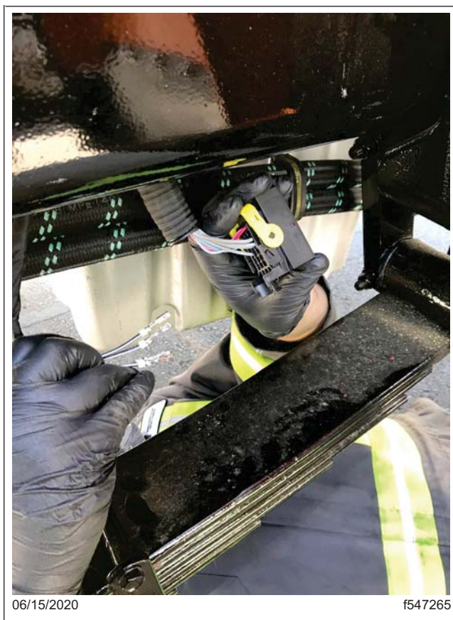
Fig. 18, MCM 21-Pin with New Terminals
