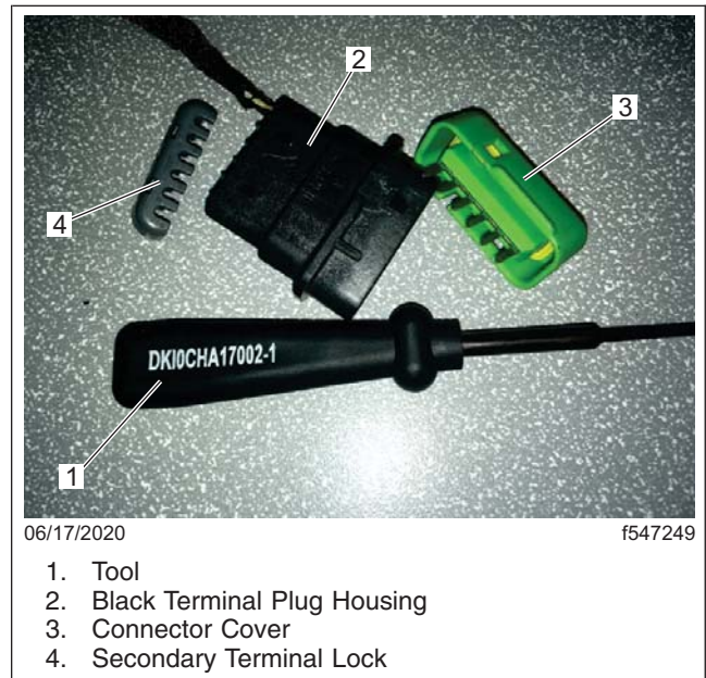
Fig. 7, Splice Pack Removal
