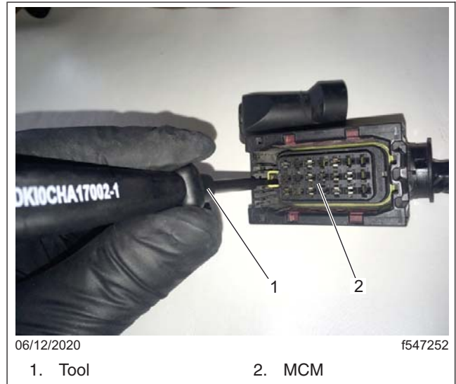
Fig. 13, Releasing the MCM Secondary Lock
