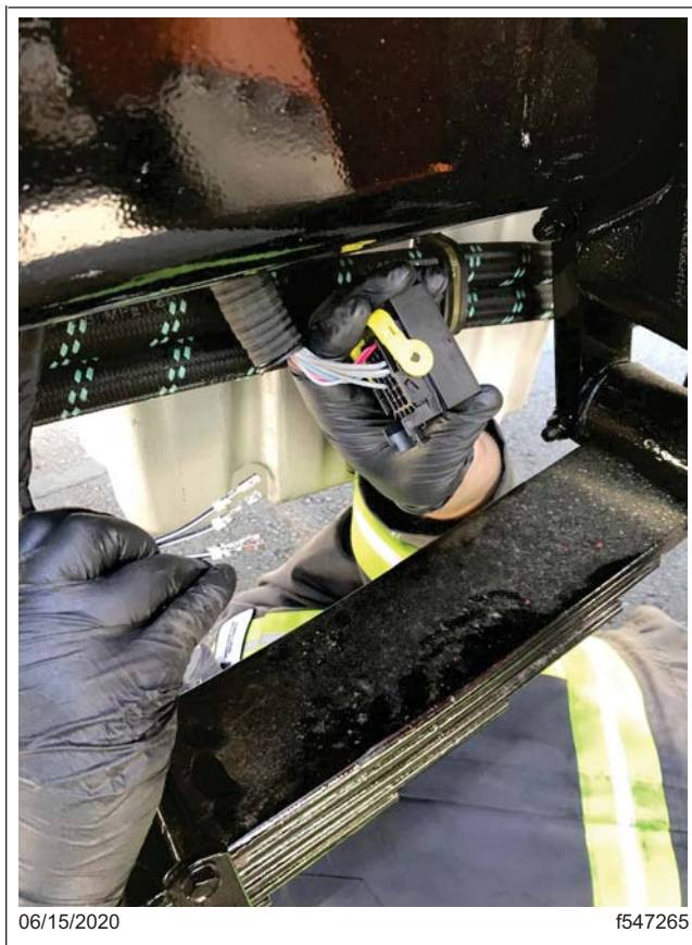
Fig. 18, MCM 21-Pin with New Terminals
