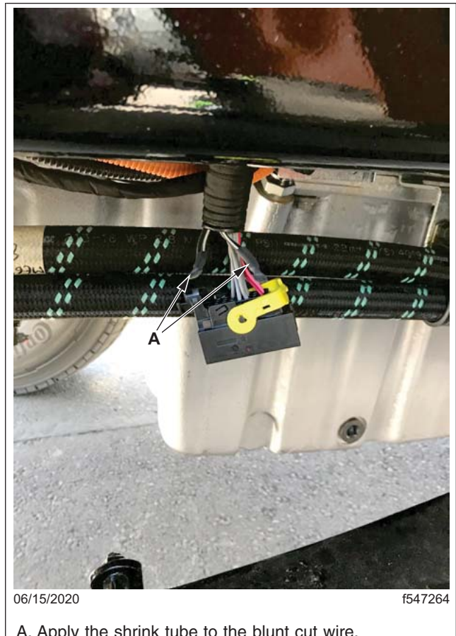
Fig. 16, Shrink Tube Applied
