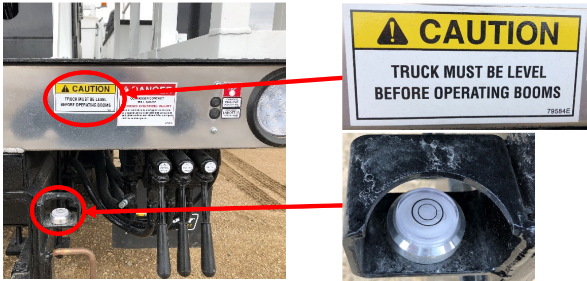
Figure 2. This bulletin does not apply if slope indicator and decal require the unit to be level.
