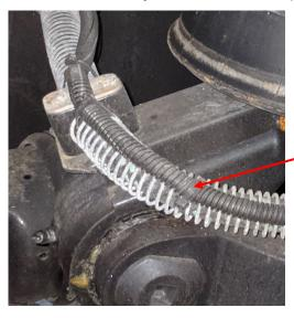
Secure the ABS sensor harness to the front brake hose using cable ties, 19-11-258
