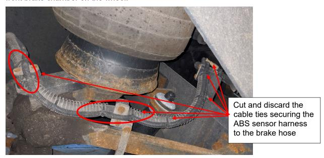
Remove the three clamps (A-post clamp, middle clamp, and frame bogie clamp), plates, and hardware securing the brake hose to the axle. Save the clamps and plates. Discard the hardware. Make sure not to remove the bracket securing the middle clamp.
