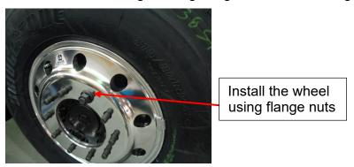
Torque the nuts to 450-500 Ft-Lb in the sequence shown below.
