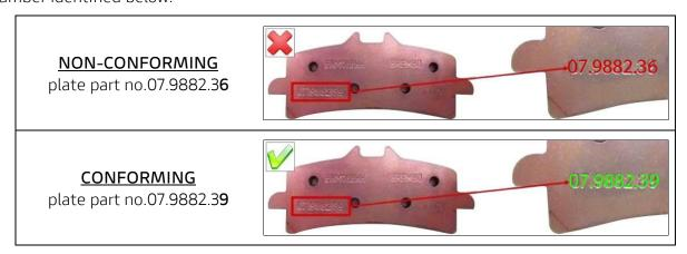
The part number of the conforming front brake pad set required to order in DCS is 61341461A.
