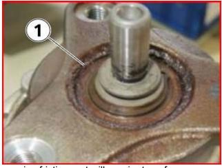
Output flanges with friction rust (1). Flanges with excessive friction rust will require transfer case replacement.
