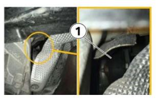
1. Raise the vehicle and determine which style flex disc is installed (1).
