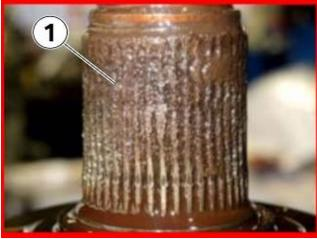
Flange and output shaft **with** friction rust damage (1). The transfer case will need to be replaced (with new flex disc).
