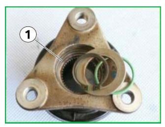
Typical output flanges without friction rust build up (1). No further repair is necessary if there is no friction rust around the splines of the output flange.
