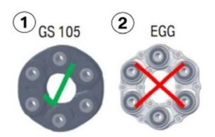
No further action is required if a black, corded rubber style (GS105) flex disc is installed (1).
