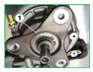
Typical output flanges without friction rust build up (1).
