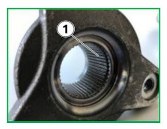
Typical flange and output shaft **without** any friction rust damage (1). Reinstall the flange (with new radial oil seal, O-ring and retaining ring) and reassemble the vehicle with new flex disc.
