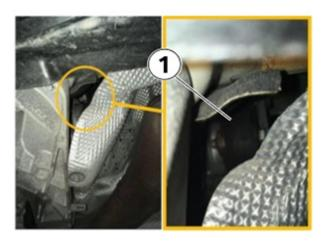
1. Raise the vehicle and determine which style flex disc is installed (1).
