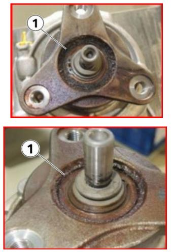
If rust build up cannot be determined by visual inspection, the flange will need to be removed for further diagnosis.
