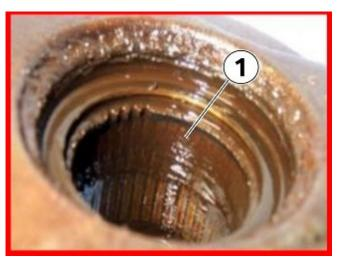
Flange and output shaft **with** friction rust damage (1). The transfer case will need to be replaced (with new flex disc).
