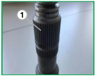
Typical flange and output shaft **without** any friction rust damage (1). Reinstall the flange (with new radial oil seal, O-ring and retaining ring) and reassemble the vehicle with new flex disc.
