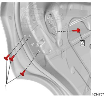
**IMPORTANT**: The rear door latch fasteners (1) are one-time use components. Replace the six (three per side) rear door latch bolts with new bolts when reinstalling the latch assemblies. The inner attachment fastener (2) can be reused.
