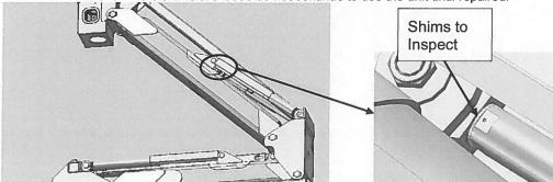
2. From the lower controls raise the lower lift boom to 45 degrees and look under the cylinder cover at the shims at the rod end. If the shims are loose do not continue to use the unit until repaired.
