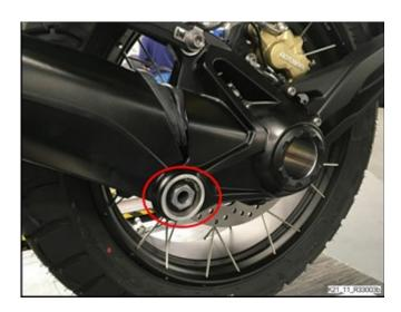
Figure 1: Affected pivot pin (circled)
