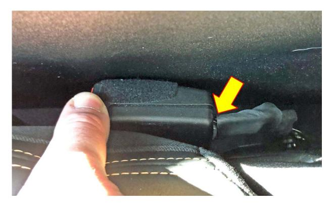
Verify visually if the hall switch remains in the correct position. Movement UP TO 3 mm is acceptable.
