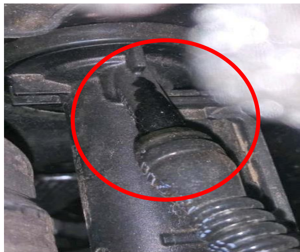
SAMPLE of Leak/Seepage
