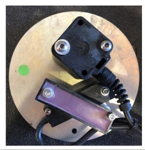
This bulletin does **NOT** apply if the Light colored potting visible on top sensor only
