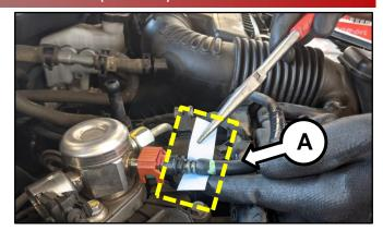
3c. If moisture is NOT present, turn the engine OFF and proceed to step 4 to tape and cable tie the fuel line.
