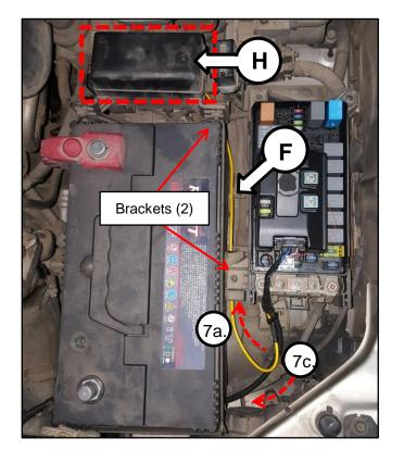
Remove the ABS2 20A fuse in the 8. gasoline box.
