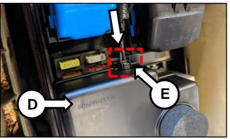
5. Connect the opposite end of the cable (E) to the battery negative terminal as shown.
