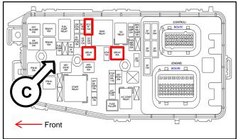
Install the relay block (D) to the junction box (C). Be sure to align the bottom connections to the removed fuses on the junction box.
