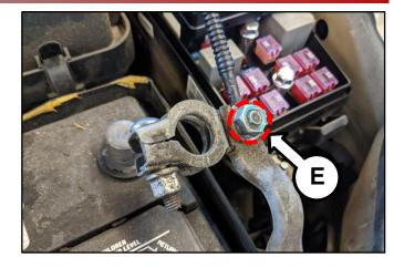
6. Re-connect the negative (-) battery terminal to the battery post and route the relay block cable (E) around the junction block.
