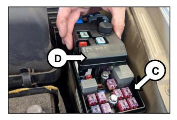
4. Connect the supplied cable (E) from the kit to the back of the relay block (D).
