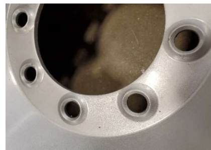
Properly Manufactured Wheel Correct Lug Nut Seat
