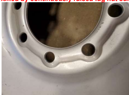
Defective Supplier Wheel Improper Lug Nut Seat and Potential Cracks
